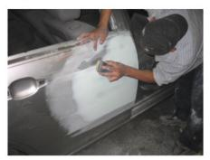
Step 5: Body Repairs are Completed
